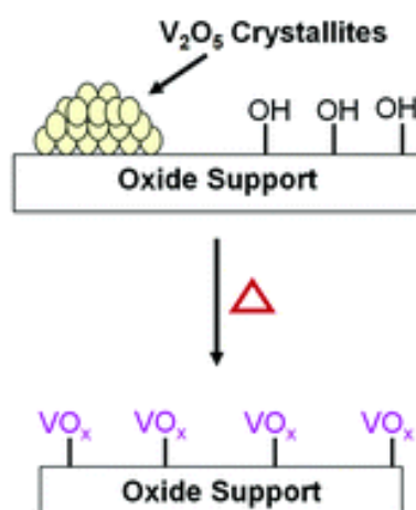
Figure 2.2: Schematic representation of \text{V}_2\text{O}_5 nanoparticle formation on top of a surface vanadia monolayer on an oxide support (Wachs, 2013)
