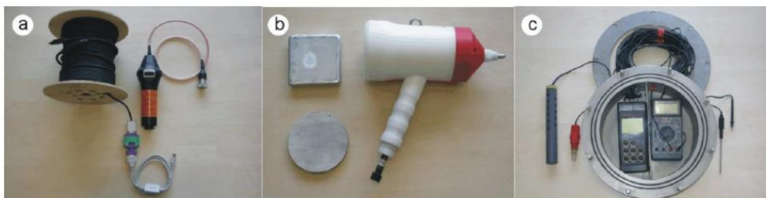
Figure 2.16: Monitoring the corrosion of steel-sheet piles using ultrasound and corrosion potential measurements
