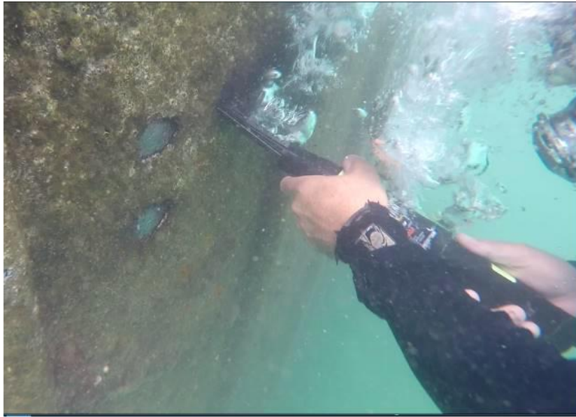
Figure 2.18: Underwater cleaning at the measurement points Source: Solorzano (2018)
