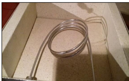
Figure 4-15: Coiled and packed column tube with a DES stationary phase
