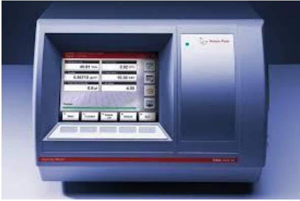
Figure 4-1: Photograph of Anton Paar DSA 5000 M Densitometer (taken from Anton Paar guideline book)
