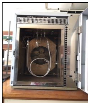
Figure 4-16: Installed column in GLC
