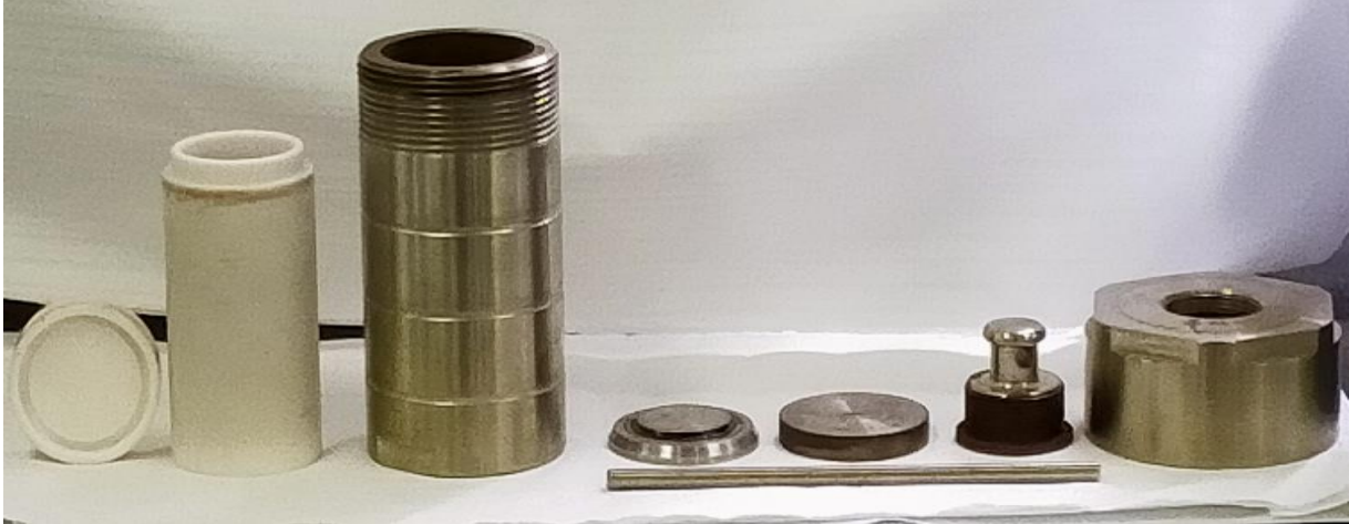
Figure 4-5 stainless steel Teflon-lined hydrothermal reactor
