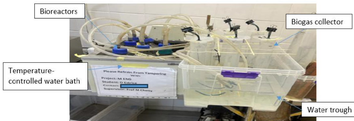
Figure 3-3: BMP experimental set-up.
