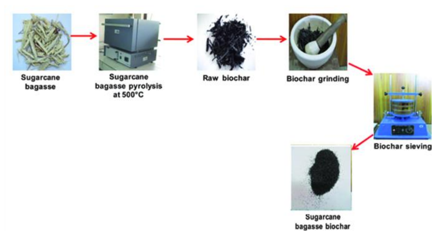
Figure 3-1: Biochar synthesis process outline.
