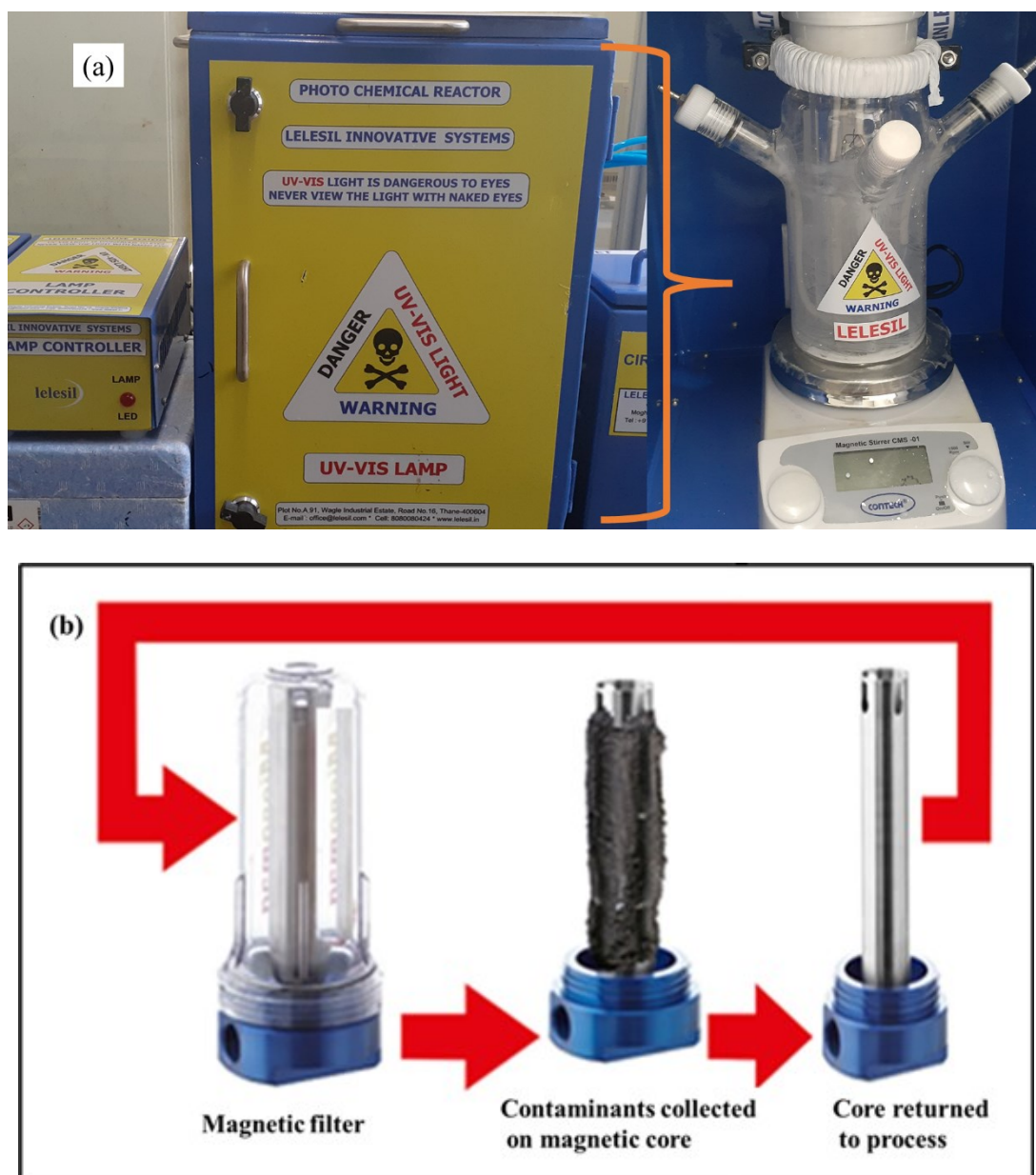
Figure 4.1: Cross-section view of (a) photocatalytic reactor setup and (b) magnetic filter
