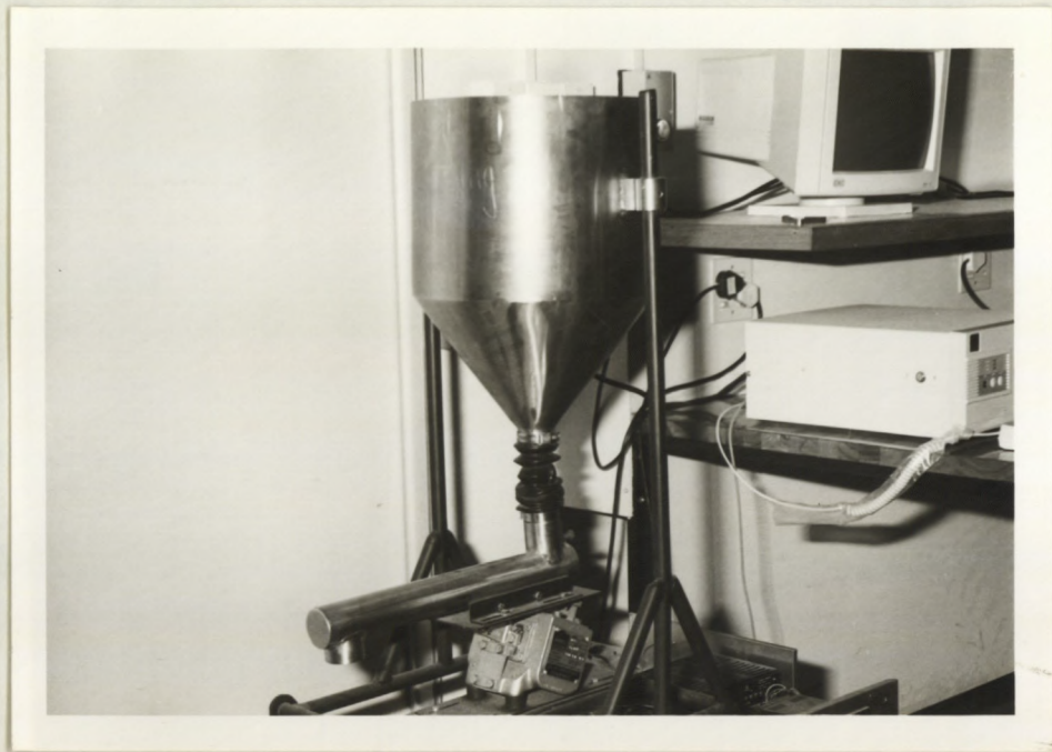
Fig 3. Photograph showing the hopper and feeder pipe.
