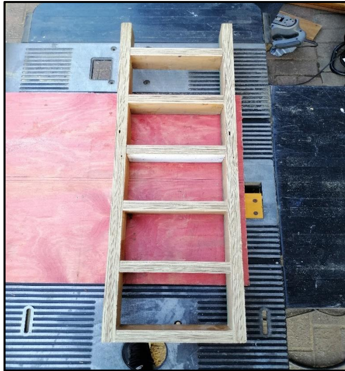
Figure 4. 6: Construction of brick mould
