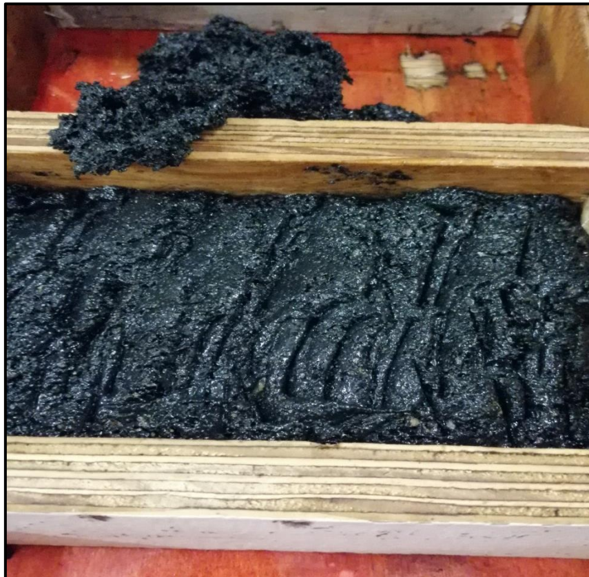
Figure 4. 8: Movement of composite to brick mould
