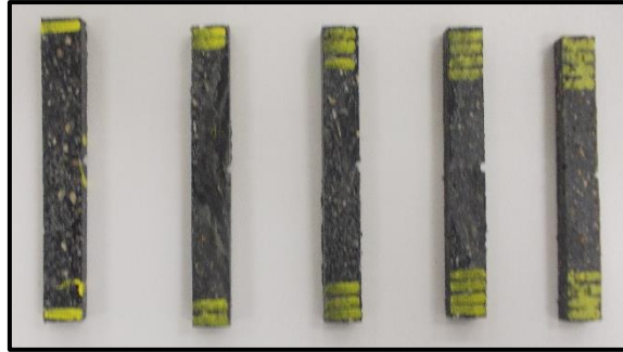
Figure 4. 12: Impact samples- 85mm (L) x 12.7mm (W) x 6mm (T) with a notch of 2mm depth was machined on all the specimens.
