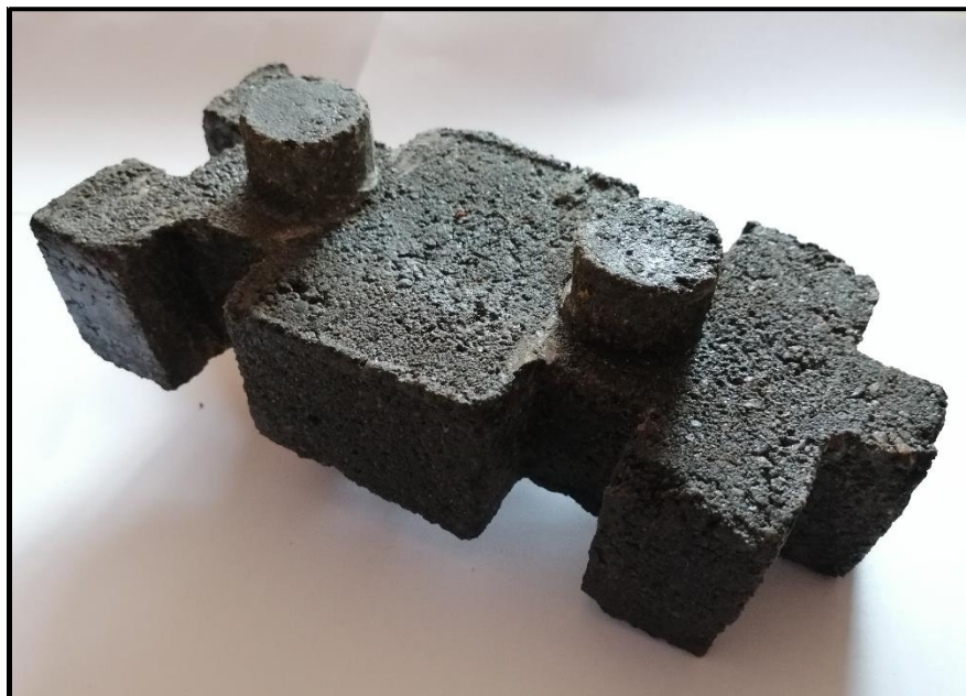
Figure 7. 6: Sample of the innovative interlocking plastic-sand brick using pressure fit
