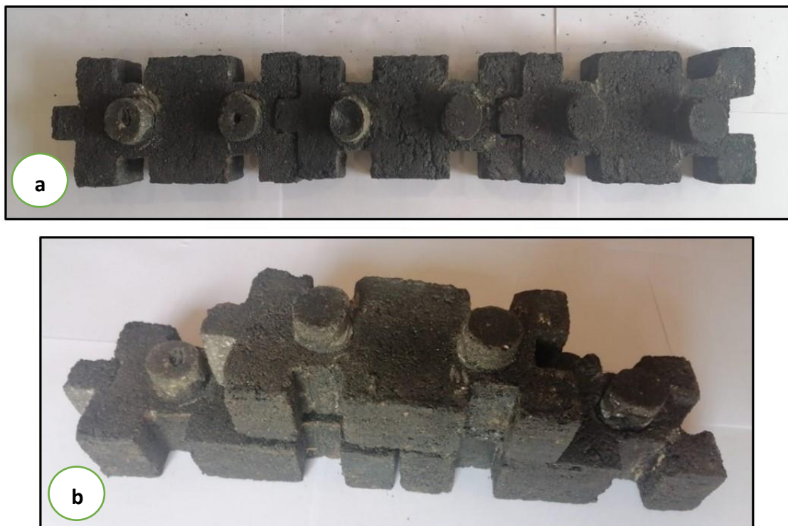
Figure 7. 8: a) Horizontal and b) vertical straight line walling
