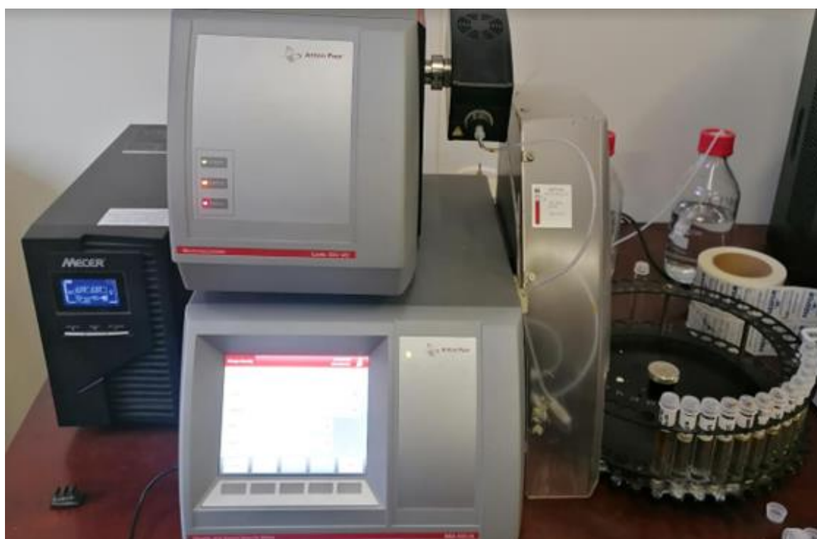
Figure 4.1: Photograph of the Anton Paar DSA 5000M coupled with microviscometer Lovis 2000ME and X sampler 452.
