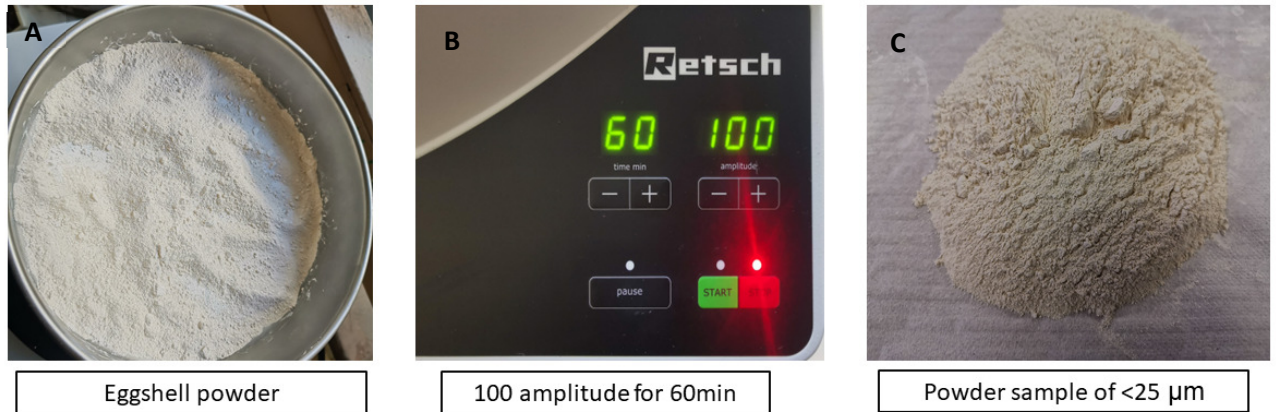
Figure 3. 3: Mechanical sieving process: (A) powder in a sieving mesh; (B) milling condition; and (C) sieved eggshell powder
