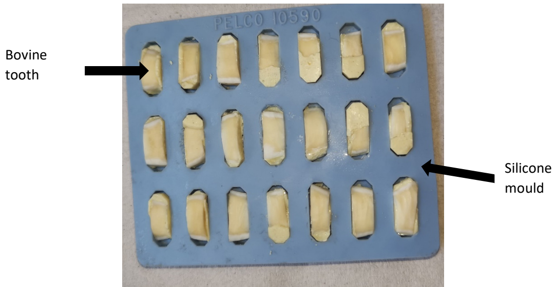
Figure 3. 9: Showing bovine embedded in silicone mould
