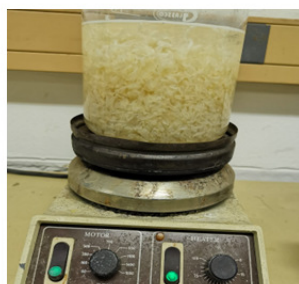
Heating at 80 °C for 20 min
