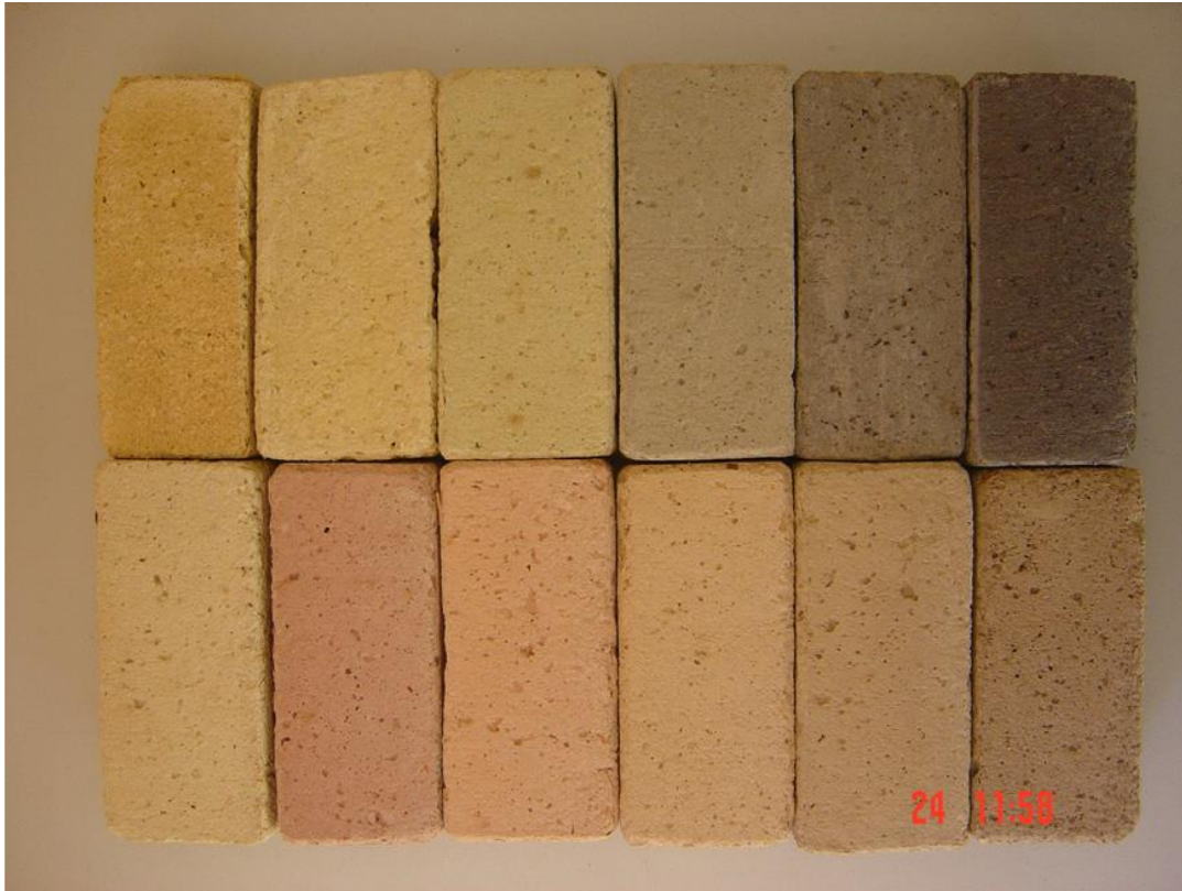
Figure 2. 5: Timbercrete in various colours, sizes and shapes. Adopted from (Timbercrete Pty. Ltd 2015)
