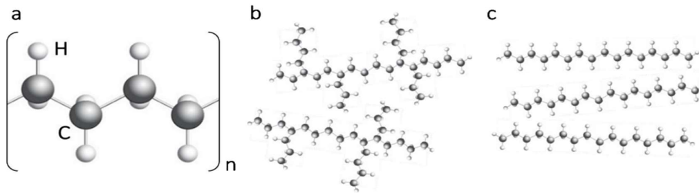
Figure 1: (a) Simple molecular structure of polyethylene includes no ionic bonds or polar groups typical for other polymers. (b) Branched structure of LDPE molecules compared to the linear-chain structure typical for HDPE and UHMWPE (c) [14].
