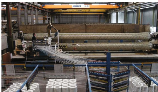
FIGURE 10: Helical filament winding used in Composite Pipes Industry (CPI), Oman [140].
