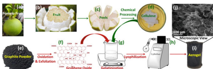
Fig. 3 a Pomelo fruit, b peeling of pomelo fruit, c peels, d cellulose extracted by chemical processing of fruit waste (peels). e Graphite powder, f representative chemical structure of GO, which is prepared by severe oxidation and exfoliation of graphite powder. g Gelatinization of GO with cellulose into a hydrogel. h Lyophilization of cellulose-GO hydrogel into CGA composite aerogel. i Digital photograph of CGA aerogel. j Microscopic view of aerogel demonstrating the porous structure. Reprinted with permission from [40]. Copyright (2022), Elsevier
