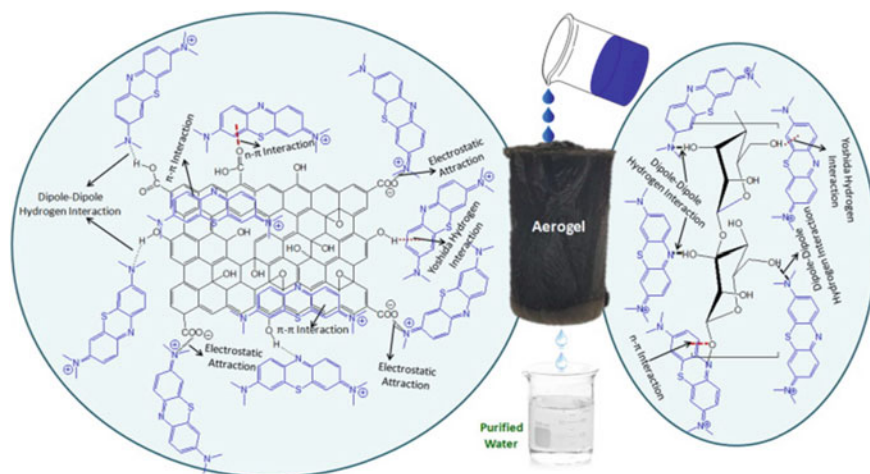
Fig. 4 Schematic representation of plausible interactions between active surface sites/chemical functionalities of CGA and MB dye molecules. Reprinted with permission from [40]. Copyright (2022), Elsevier
