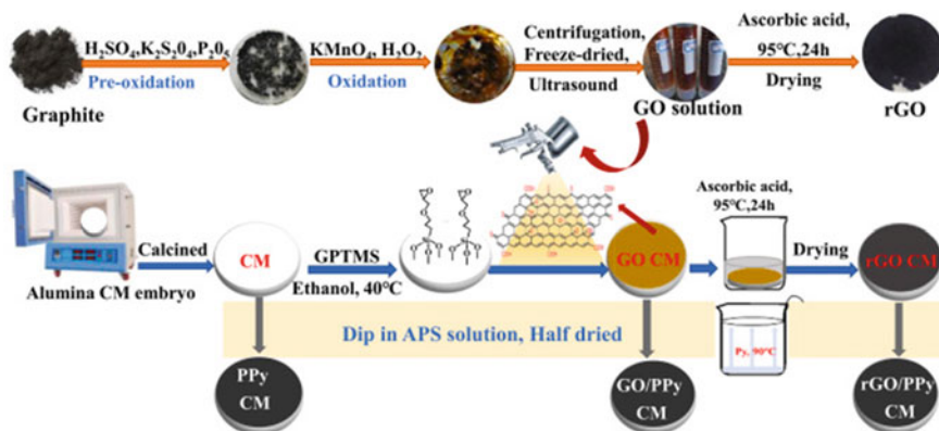
Fig. 13 Schematic diagram of the preparation process for GO, rGO, and conductive membranes. Reprinted with permission from [48]. Copyright (2022), Elsevier
