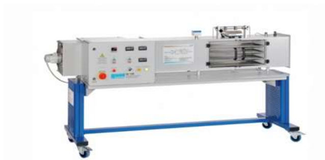
Figure 3.2: Gunt Hamburg air-convection drier (CE 1300 model)
