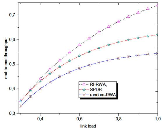
Figure 8: End to end throughput as a function of link load
