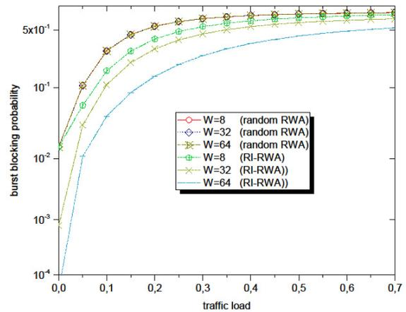
Figure 3: Blocking probabilities versus link c load
