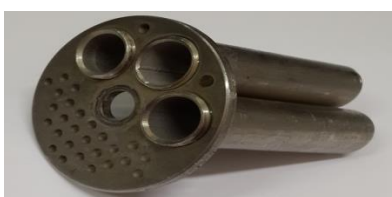
Figure 1 – Type 1 (cylindrical downcomer)
