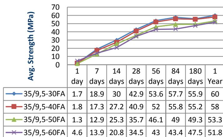
**Figure 1: Compressive strength results of 35MPa mixtures**
